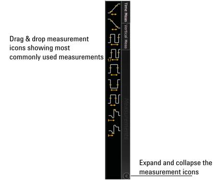
Figure 20 Drag & Drop measurements
