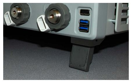
Figure 4 Flip-Out tabs under front feet
