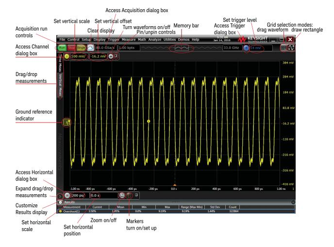
Figure 10 calls out the areas and controls of the user interface.
