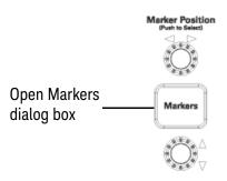
Figure 19 Front panel measure controls
