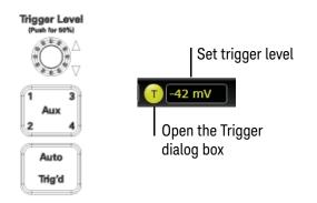
Figure 18 Trigger controls and indicators
