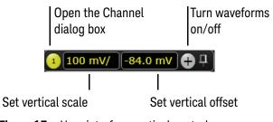
Figure 17 User interface vertical controls
