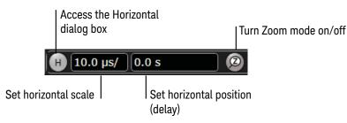
Figure 15 User interface horizontal controls
