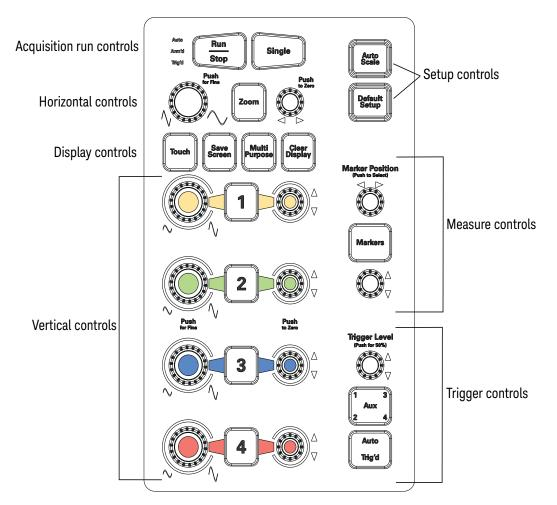
Figure 9 Infiniium V-Series oscilloscope front panel
