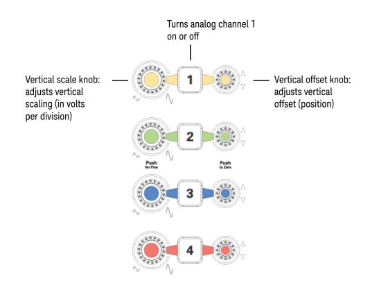
Figure 16 Channel keys and vertical scale and offset knobs
