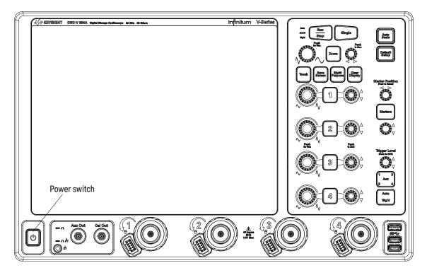
Figure 5 Turning On the oscilloscope
