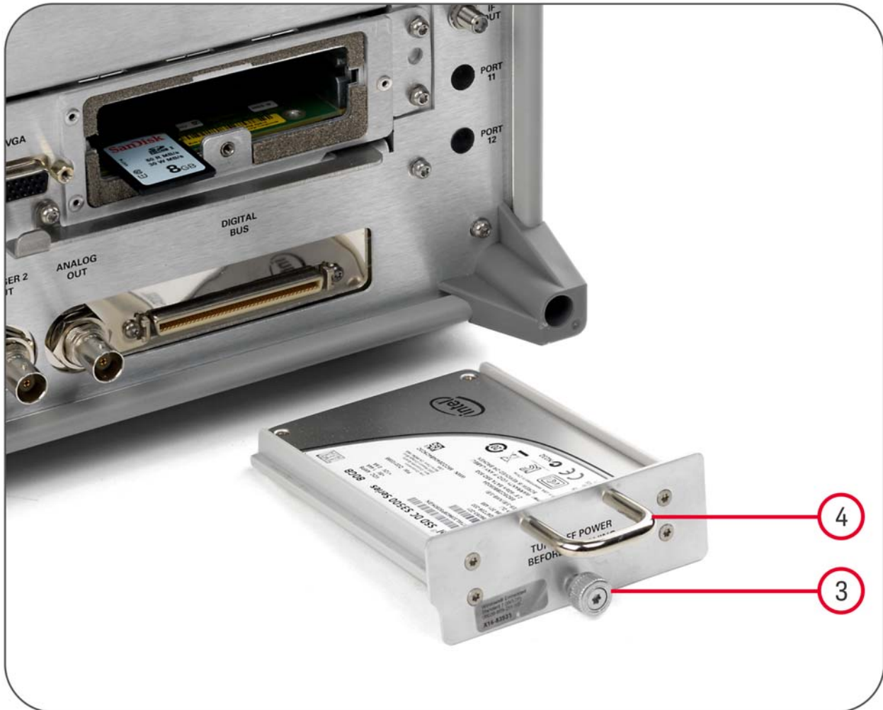
Figure 6-2 Removable Disk Drive Unit fully extracted
