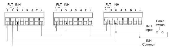
As shown in the figure, when the Fault outputs and Inhibit inputs of several mainframes are daisy-chained, an internal fault condition in one of the mainframes will disable all of them without intervention by either the controller or external circuitry.
