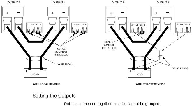
To program outputs connected in series, first program the current limit of each output to the total desired current limit point. Then program the voltage of each output so that the sum of both voltages equals the total desired operating voltage. The simplest way to accomplish this is to program each output to one half of the total desired operating voltage.
