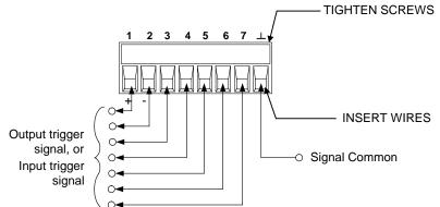
The digital control connector accepts wires sizes from AWG 14 to AWG 30. Note that wire sizes smaller than AWG 24 are not recommended. Disconnect the connector plug to make your wire connections.
