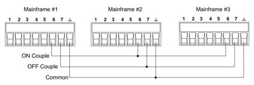
Only *two* of the digital connector pins on each mainframe can be configured as "ONCouple" and "OFFCouple" on each synchronized mainframe. The designated pins will function as both an input and an output, with a negative transition on one pin providing the synchronization signal to the other pins.
