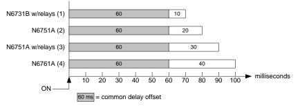
Since there will be an additional delay due to the common delay offset, you will need to account for the additional delay time. As shown in the previous example, if you program a common delay of 60 ms and user-programmed delays of 10 ms, 20 ms, 30 ms, and 40 ms for output channels 1 through 4, the actual output delays from the "on" event will be 70 ms, 80 ms, 90 ms, and 100 ms respectively.
