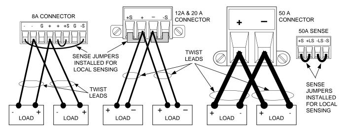
This minimizes mutual coupling effects and takes full advantage of the power system's low output impedance. Keep each pair of wires as short as possible and twist or bundle them to reduce lead inductance and noise pickup.
