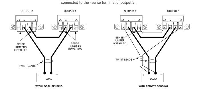
The following figure shows the connections for 50A power modules.
