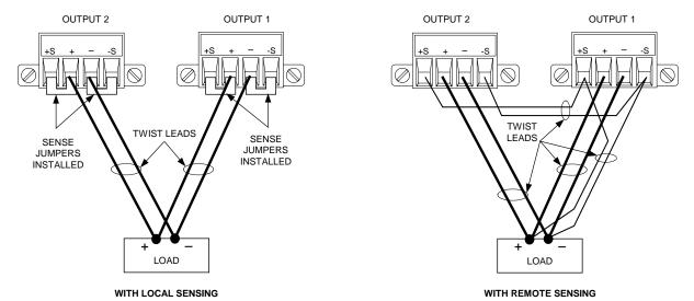
The following figure shows the connections for 50A power modules.
