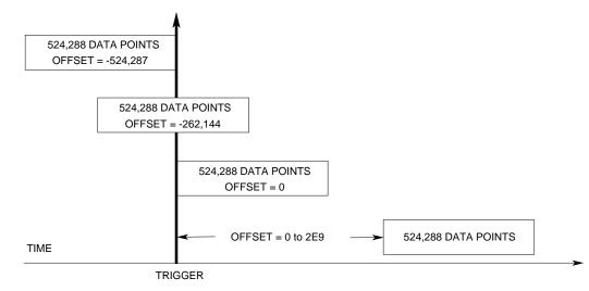
To offset the beginning of the acquisition buffer relative to the acquisition trigger, use:
