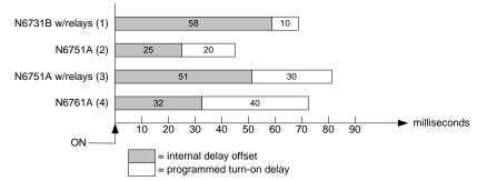
To synchronize power modules with *different* minimum delay offsets as shown above, you can specify a *common* delay offset parameter. By setting the common delay offset to be greater than or equal to the largest minimum delay offset, you can synchronize the programmed turn-on delays as shown in the following example.
