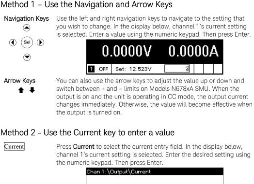
Current 2.0000If you make a mistake, either use the *the backspace key to delete the* NOTE number, press Back to back out of the menu, or press Meter to return to meter mode.
