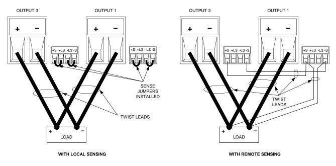
The following figure shows the paralleled connections for N678xA SMU power modules. Note that remote sensing is not normally used in Current Priority mode.
