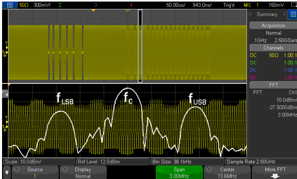
Figure 5. Performing a gated FFT measurement on NFC-A load modulation.
