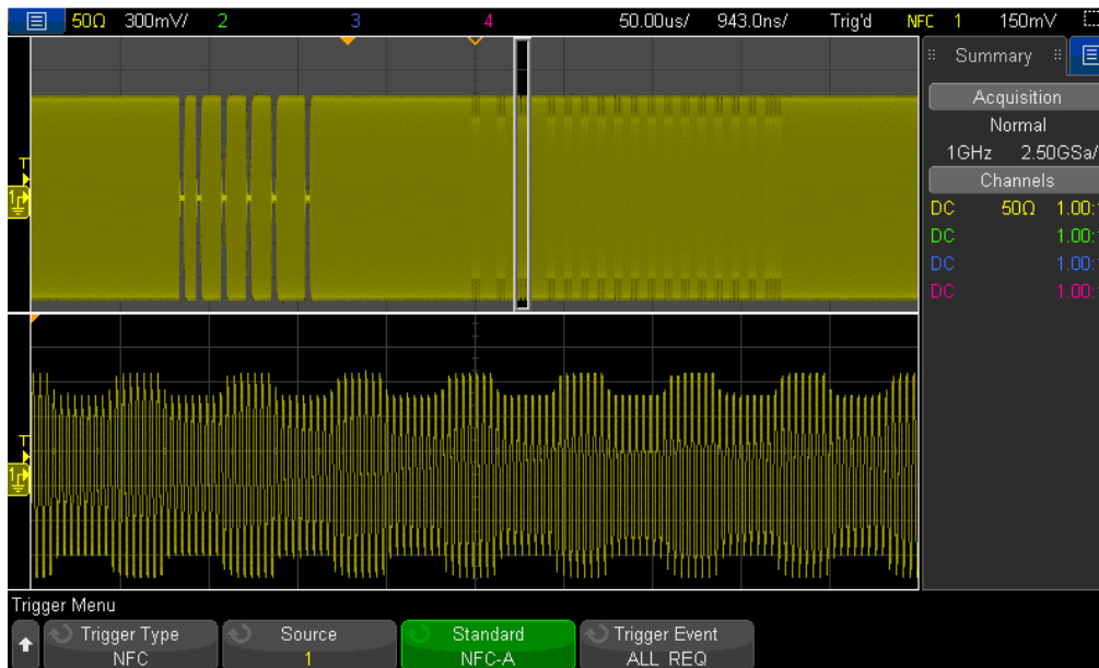
Figure 4. Windowing on exactly eight cycles of modulation.
